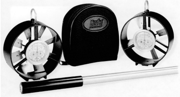
Figure 3.16 The conventional rotating vane anemometer (Birams type) consists of an aluminum vane impeller with a mechanical gear train driving a series of three dials that read 100, 1000, and 10,000 ft (30.5, 305.0, and 3050.0 m). The instrument is equipped with a zero-reset lever and a lever to activate the instrument. This unit has a 4-in. (10-cm)-diameter frame and has a useful range of 100–5000 fpm (0.51–25.5 m/s). It is available from several manufacturers. (Courtesy of Davis Instrument Manufacturing Co.)
