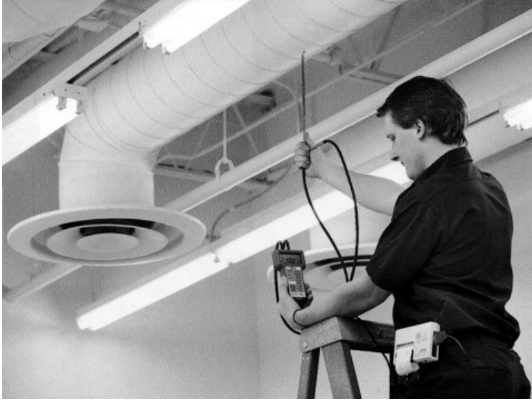
Figure 3.8 Microprocessor-based system using electronic pressure transducer for direct Pitot-static velocity measurements as shown here with averaging and storage capability. The transducer has a measurement range from -15 to 15 in. \text{H}_2\text{O} ( 3735 Pa). A belt-mounted printer permits one person to conduct and record all measurements. (Courtesy of TSI Inc.)
