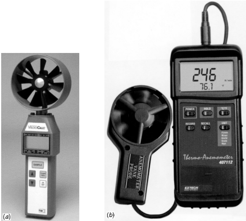
Figure 3.17 A new generation of electronic-based rotating vane anemometers has improved range and accuracy. (a) This series of instruments is available with a 4-in. (100-mm) or a 1.4-in. (35-mm) rotating vane sensor in an integral design as shown or with a telescopic probe head. It displays average, maximum, and minimum values; calculates flow; and is available with data logging capability. (Courtesy of TSI, Inc.) (b) This anemometer has a 2.83-in. (72-mm) rotating impeller with a ball bearing suspension and a 39-in. (1-m) cable and records maximum, minimum, and average values with recall functions. It has a built in serial interface with optional data acquisition software and data logger for subsequent analysis. (Courtesy of Extech Instrumentation Corp.)
