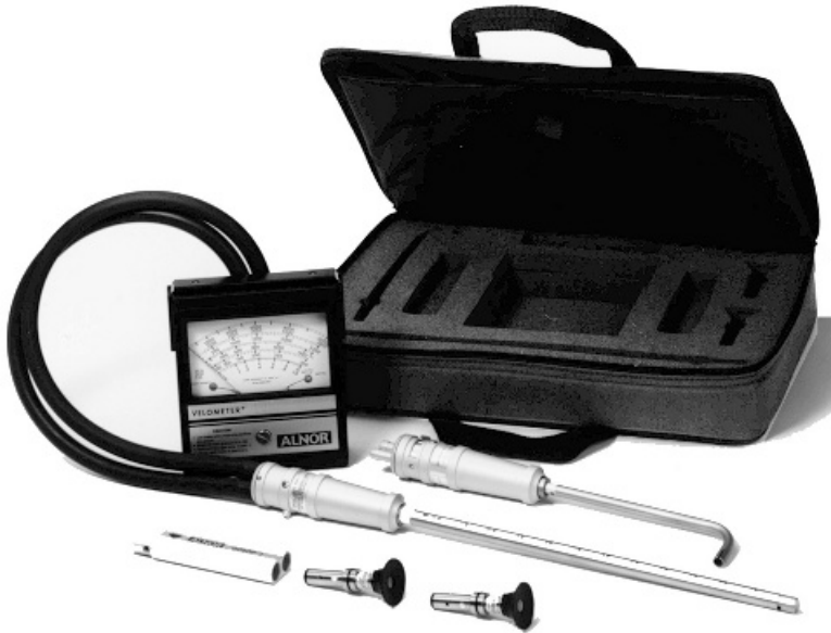
Figure 3.24 (a) The basic swinging vane instrument (Alnor Model 6000). Applications include (b) a low-velocity probe for air velocity measurements in plane of hood opening or (c) a Pitot probe with a diameter of \frac{1}{2} in. (1.27 cm). Since it does not have the 90^\circ bend of the pitot, it requires only a slightly oversized hole. The advantage of this probe is that the velocity may be read directly from the meter. The device is not a primary standard and requires calibration by a standard Pitot–static tube. Also shown is (d) a probe for measuring delivery from diffusers. By measuring the diffusers throat velocity the delivery can be calculated using the manufacturer's k factor. (Courtesy of Alnor Instrument Company a Division of TSI, Inc.)
