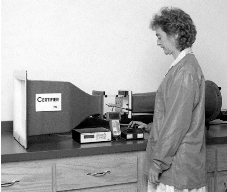
Figure 3.35 A calibration tunnel designed for small probes such as heated elements. (Courtesy of TSI, Inc.)
