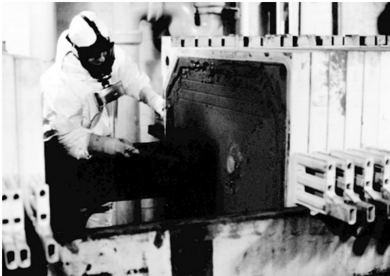
Figure 6.32 Dropping product from plate and frame filter.
