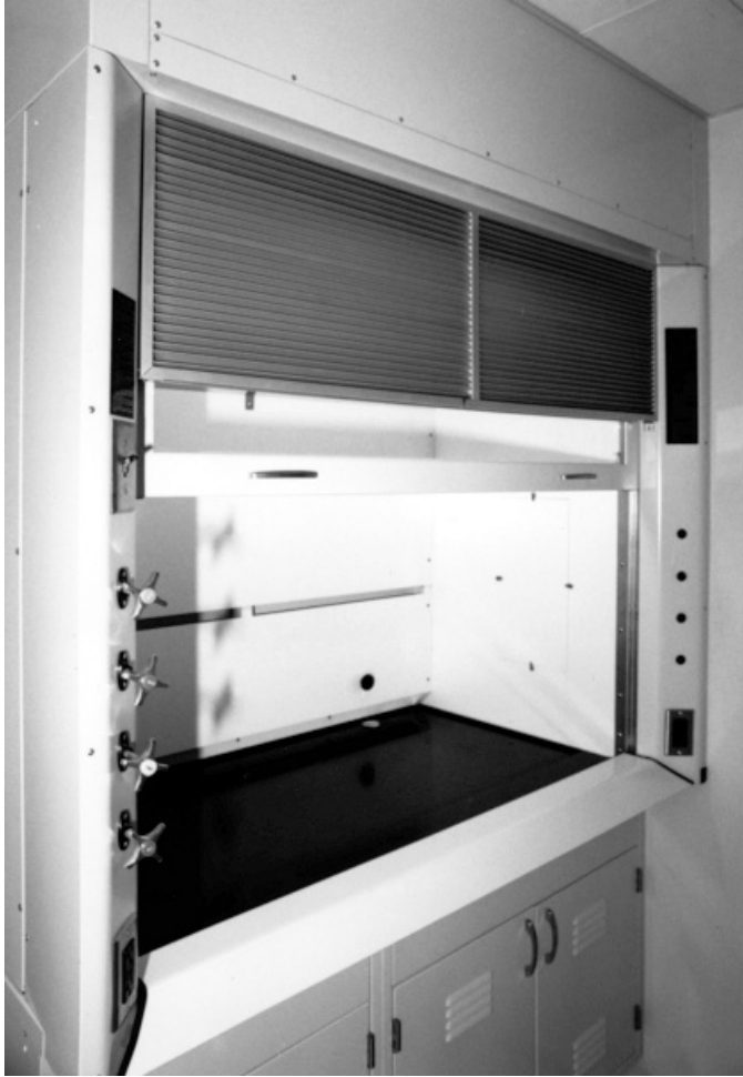
Figure 7.8 A modified constant volume/by-pass vertical sliding sash hood that incorporates the various design features, including airfoil elements, bypass feature, and multiple rear slots. (Courtesy of Fisher Hamilton LLC.)
