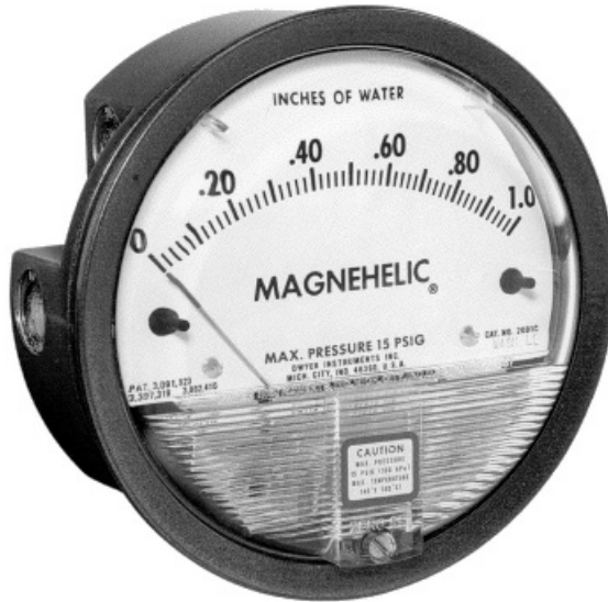
Figure 3.7 Magnehelic devices are available for a range of pressures and are useful for measuring velocity pressures as low as 0.05 in. H_2O (12.46 Pa). These sensors are convenient for field use in that they do not require leveling, are easily zeroed, and do not use fluids. Since they are not primary standards they do require periodic calibration, but this is easily done with a conventional manometer. These devices are commonly used to monitor airflow continuously at individual hoods using the hood static suction measurement technique described in Section 3.5. (Courtesy of Dwyer Instruments, Inc.)
