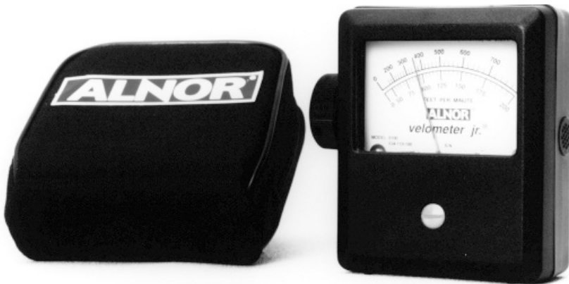
Figure 3.26 A simple and inexpensive adaptation of the swinging vane anemometer designed to monitor face velocity at simple hood openings. (Courtesy of Alnor Instrument Company a Division of TSI, Inc.)
