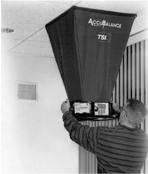
Figure 3.25 Canopy device, that can be positioned over the HVAC diffuser and directs the supply air past a swinging vane instrument. The device is calibrated directly in \text{cfm} ( \text{m}^3/\text{s} ). This procedure is more accurate than the probe technique, which measures diffuser throat velocity. (Courtesy of TSI, Inc.)
