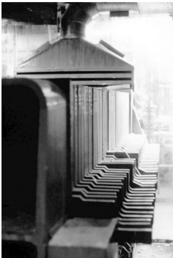
Figure 6.33 Ventilation of plate and frame filter enclosure based on rigid sliding panels or plastic curtains.
